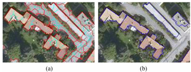
Fig. 7. Determination of final buildings: Three buildings (left) are approximated by the recursive MBR of level 2 and other two buildings (right) are rectangular. Their RMBR scores are, respectively, 0.87, 0.91, 0.84, 0.93, 0.81 (from left to right). The value of T_B is chosen as 0.8. (a) Segmentation result. (b) Final building.
