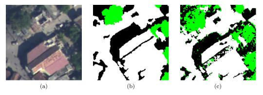
Figure 4.4: Decision making: (a) input image, (b) ground truth, (c) detected shadow/vegetation by maximizing the pignistic probability function.
