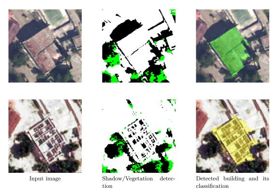
Figure 7.3: Change detection on building states: the first line represents a constructed building detected from NOAA aerial image (of time n); the second line represents the same building under construction detected from Worldview-2 satellite image (of time n+1) of Jacmel datasets. Hence, this building is classified as building under reconstruction between two different times.
