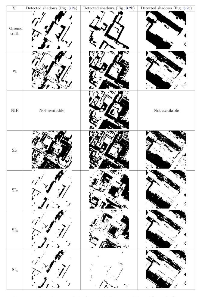
Table 3.3: Resulting shadow masks by Otsu thresholding method from different SIs for images in Fig. 3.2
