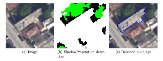
Figure 6.12: A building is not detected since its shadow can not be detected.
