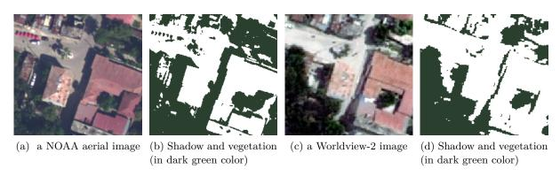
Figure 3.8: Illustration of shadow/vegetation detection using the luminance with two images from Jacmel dataset
