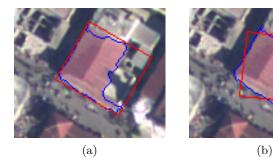
Figure 5.13: Building with protrusion artifact: (a) Building region (whose boundary is delineated by blue line) and its minimum bounding rectangle (red line). (b) Building region and the fitted rectangle estimated by discrepancy method.
