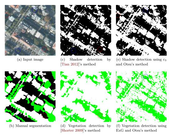
Figure 3.5: Sequential shadow/vegetation detection from a BD ORTHO® image.
