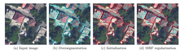
Figure 5.10: Experimental results of MRF-based region classification. Regions are separated by cyan lines and clusters are separated by red lines.
