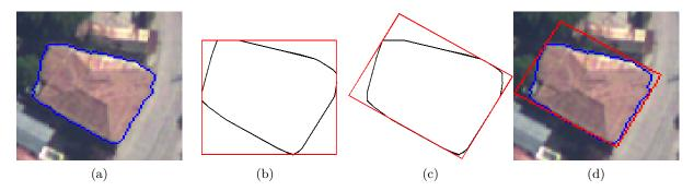
Figure 5.12: Illustration of the MBR estimation [Toussaint 1983]: (a) Object and its boundary (in blue), (b) convex hull and one bounding rectangle test (in red), (c) bounding rectangle with minimum area (in red), (d) object and its MBR
