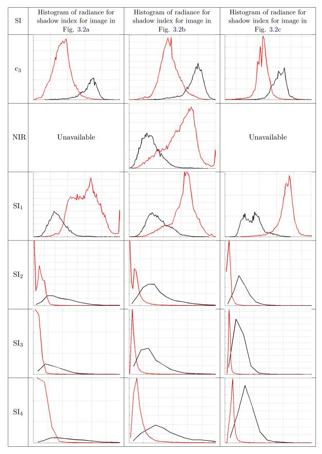
Table 3.2: Different shadow indices (first column) and histogram of radiance for shadow indices for images in Fig. 3.2. The black curve corresponds to shadow, the red curve corresponds to non-shadow. The overlaps between the shadow and non-shadow histogram of  $c_3$  and  $SI_1$  are less significant than others.
