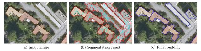
Figure 5.20: Determination of final buildings from the region growing image segmentation result: 5 buildings are detected, in which 3 buildings (left) are approximated by the recursive MBR of level 2 and other 2 buildings (right) are rectangular. These detected buildings have RMBR-scores of 0.87, 0.91, 0.84, 0.93, 0.81 respectively (from left to right). The value of  $T_B$  is chosen as 0.8.
