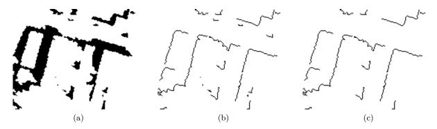
Figure 5.6: Removing shadows due to other non-building objects. (a) the shadow mask after eliminating shadows generated by vegetation, (b) potential building-shadow boundaries of (a), (c) final building-shadow boundary mask  $M_{SB}$  (black)
