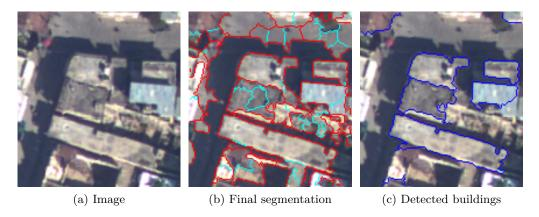
Figure 6.11: Detected building in a dense urban area. Attached buildings are separated by blue lines.
