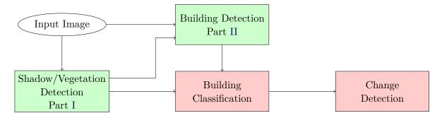
Figure 1.3: The workflow of building database update. The blocks in green are studied in the limit of this thesis.
