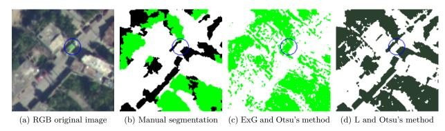
Figure 3.7: Otsu's thresholding method applied on image ExG and luminance L: (c) using only index ExG leads to classify a green and bright object as vegetation; (d) shadow regions and vegetation regions (dark green area) are well detected.
