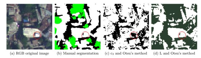
Figure 3.6: Otsu's thresholding method applied on image  $c_3$  and luminance L: (c) using only index  $c_3$  leads to classify a very bright object as shadow; (d) shadow regions and vegetation regions (dark green area) are well detected.
