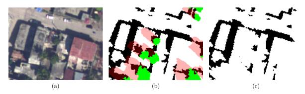
Figure 5.5: Removing shadows due to vegetation. (a) RGB aerial image, (b) The expansion regions (pink color) generated after the dilation of the vegetation objects overlaid with the shadow/vegetation map, (c) the shadow mask after eliminating shadows generated by vegetation
