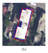
Figure 5.14: Building with intrusion artifact: (a) Building region (whose boundary is delineated by blue line) and its minimum bounding rectangle (red line). (b) Building region and the fitted rectangle estimated by discrepancy method.
