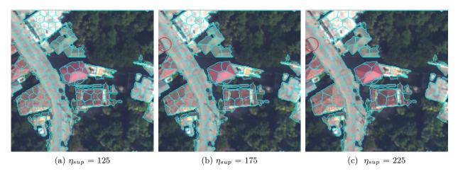
Figure 6.1: An example of oversegmentation SLIC with different values of  $\eta_{sup}$ . Low value of  $\eta_{sup}$  produces lots of regions and high value of  $\eta_{sup}$  makes the oversegmentation not adhere well to building boundaries.
