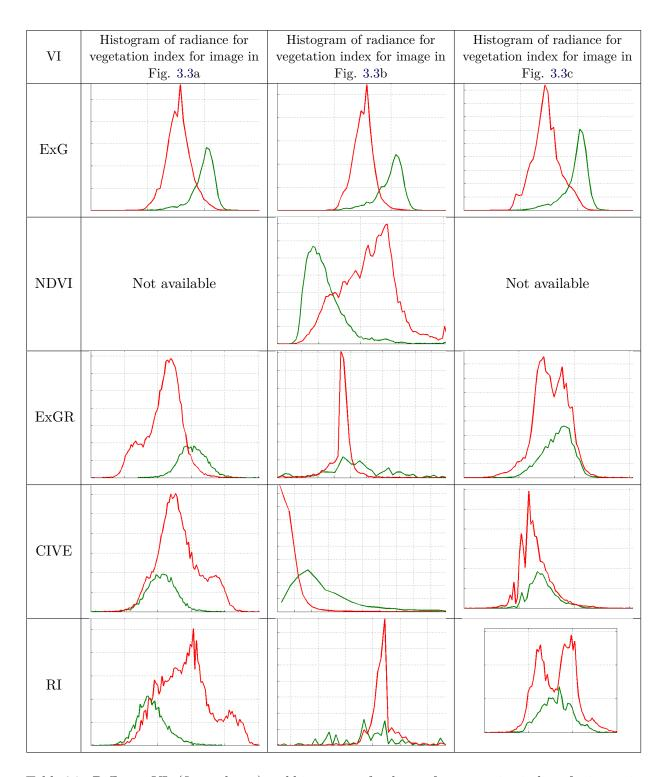
Table 3.7: Different VIs (first column) and histogram of radiance for vegetation indices for image in Fig. 3.3. The green curve corresponds to vegetation, the red curve corresponds to non-vegetation. The overlaps between the vegetation and non-vegetation histogram of ExG and NDVI are less significant than others.
