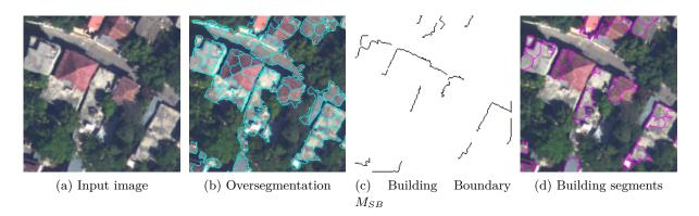
Figure 5.11: An example of building segments detection. We observe that each targeted building has one or several building segments.
